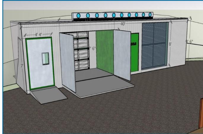
*Airwise, Buildings in a Boxes™ are standardized Airwise Structure systems. Each preconfigured package includes all electrical and mechanical equipment necessary to store, transport and support operation of a 6,000 to 70,000 sq. ft. Airwise Structure, contained in one to two modified 40' shipping containers.*
